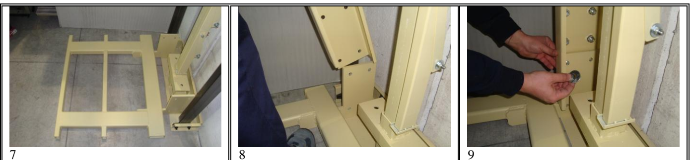
Place the base of the arch in the center of the guides
